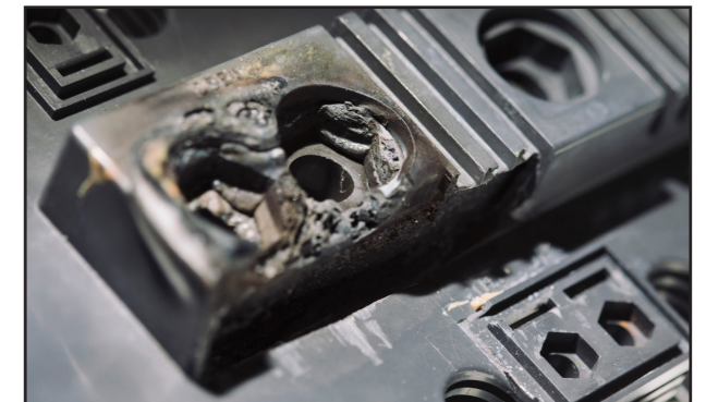
Defective power electronic packaging module
